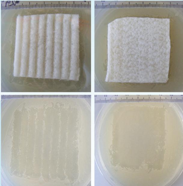
**Figure 2-** Dressing A (top left), and Dressing B (top right) on a bacterial lawn following 24hr incubation. Upon removal no growth is seen beneath Dressing A (bottom left). Distinct bacterial lines can be seen beneath Dressing B (bottom right).
