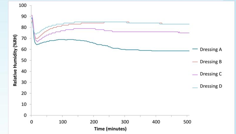
Graph three – Relative humidity measured underneath dressings over 500 minutes
