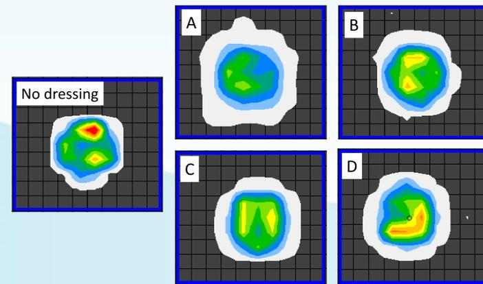
Figure one – Images of the pressure profiles recorded when a weight was applied with and without a dressing to a pressure mat. Red = high pressure, white = low pressure.
