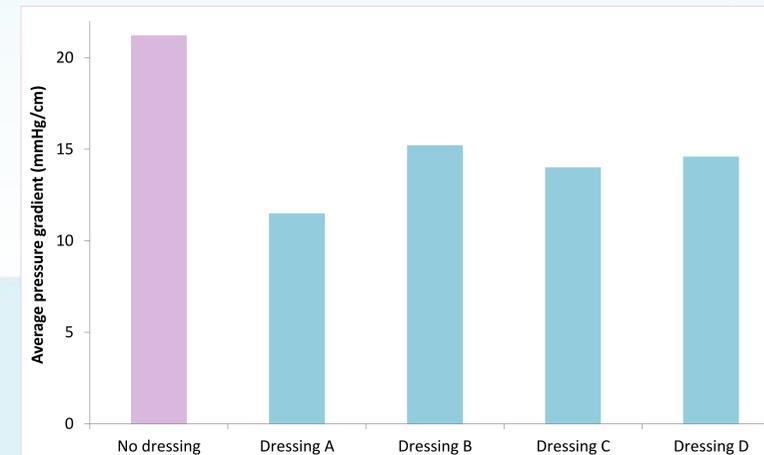
Graph two – Average pressure gradient recorded when a weight was applied with (n=3) and without (n=10) a dressing to a pressure mat
