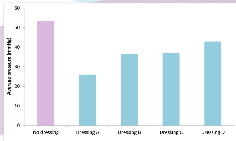
Graph one – Average pressure recorded when a weight was applied with (n=6) and without (n=10) a dressing to a pressure mat
